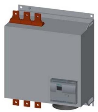
SIRIUS soft starter Values at 400 V, 40 °C Standard: 880 A, 500 kW Inside-delta: 1524 A, 900 kW 200-460 V AC, 230 V AC Screw terminals
