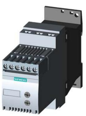
SIRIUS soft starter S00 6.5 A, 3 kW/400 V, 40 °C 200-480 V AC, 24 V AC/DC Screw terminals
